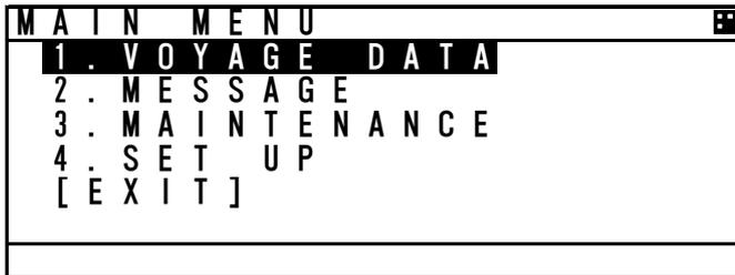
Press **▲** key or **▼** key for moving the cursor over the menu to select a desirable item. Press **ENT** key, and then the selected menu is displayed.
