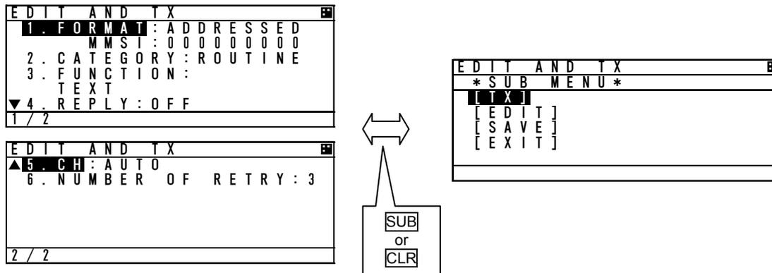
1. Press ▲ key or ▼ key in “EDIT AND TX” screen and move the cursor to a desirable item, and then press **ENT** key. The cursor is moved to a selecting portion at the right side (The above example; Press **ENT** key at the “FORMAT”, the cursor is moved to **ADDRESSED**.)
