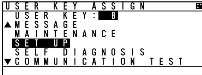
When USER KEY ASSIGN screen is displayed, the cursor is on the current setting.
