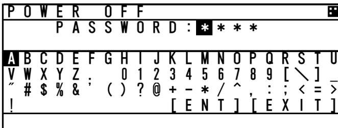
When turn off the power, press and hold **PWR/CONT** key and **DIM** key together for 1 second and then “PASSWORD” input screen is displayed. Enter 4 digits of password, select **[ENT]** and press **[ENT]** key. Password is composed of alphanumeric “A~Z” and “0~9”.
