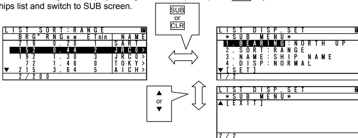
When the screen is switched from the SUB menu screen to “LIST SORT” screen, press **[CLR]** key or select [EXIT], and then press **[ENT]** key.
