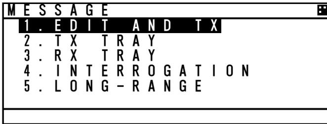
When move the cursor for selecting a desirable item in menu, press ▲ key or ▼ key. then press **ENT** key to display a screen of the selected item.
