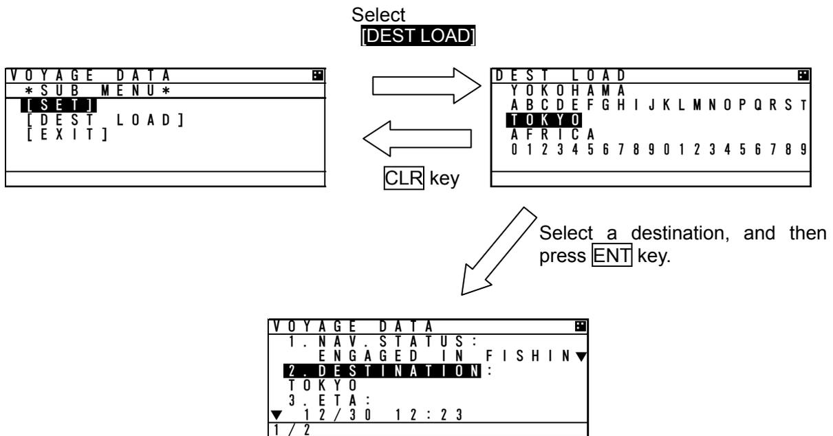
Select the destination from the list and press **[ENT]** key, then the screen is switched to “VOYAGE DATA” menu screen and the selected one is displayed at the **2.DESTINATION**.
