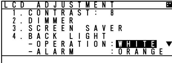
Select WHITE or ORANGE at "OPERATION" with ▲ key or ▼ key. After setting, press **ENT** key, and then the cursor move to the right side of "ALARM". Take the same procedure.
