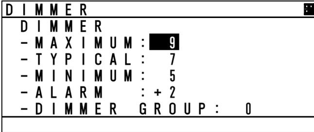
When the cursor is on the right of "MAXIMUM", the value can be adjusted. Press **▲** key or **▼** key to adjust it and press **ENT** key and then the cursor moves to the right of "TYPICAL". The value of MAXIMUM, TYPICAL and MINIMUM can be set between 1 to 13.
