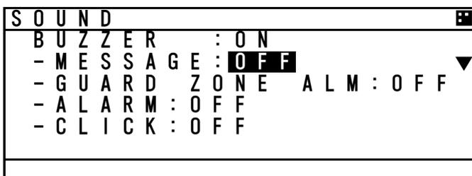
When "ON" is selected at "BUZZER", select from ON and OFF and set each of items.
