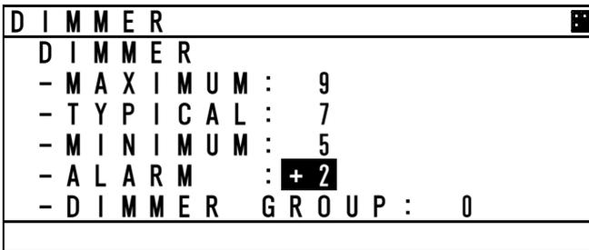
The ALARM value can be set between +1 to +9. In the case of an alarm, the current dimmer setting is altered by the value set here.
