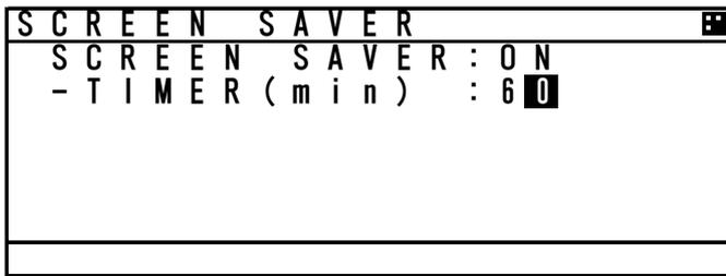
Select "ON", the cursor move to TIMER value. Set the value between 00 and 60 (minutes) with ▲ key or ▼ key and press **ENT** key.
