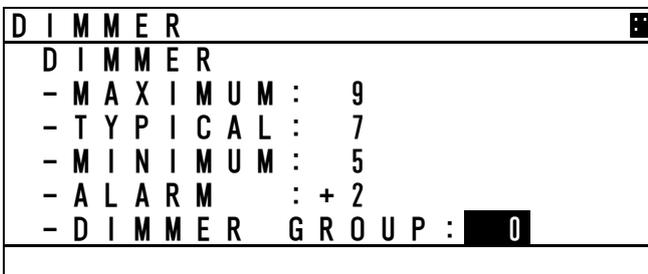
When the AIS JHS-183 connect the JRC display equipment, set a group within which dimmer control for this display unit is linked. The DIMMER GROUP value can be set between 0 to 10. Available dimmer group numbers are from 1 to 10. Unavailable dimmer group number is 0. Select the same dimmer unit within the same group. Otherwise, dimmer control cannot be linked within the group.
