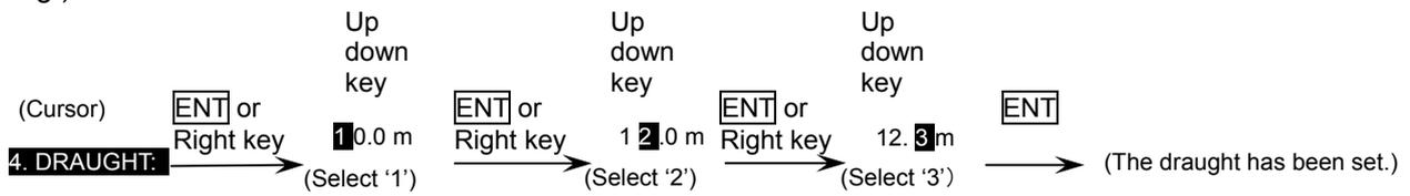
When **CLR** or left key is pressed, the cursor is moved back to 1 digit left position.
