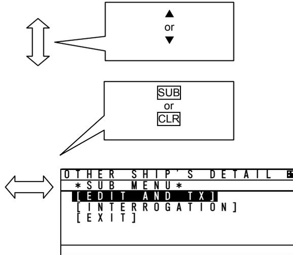
Press **[SUB]** key in order to display the Sub menu, and then the cursor can be moved with "▲"key or "▼"key.
