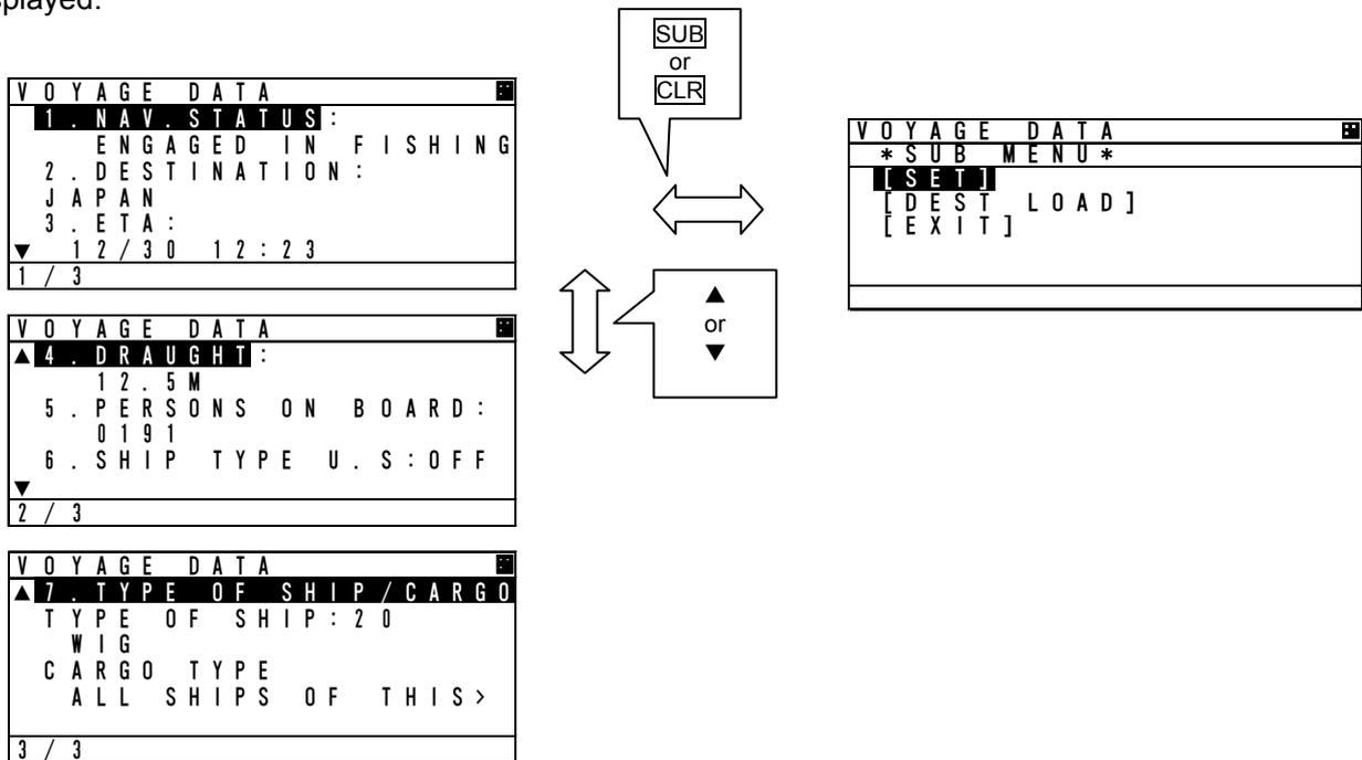
Press **▲** key or **▼** key to select a desirable setting item and press **ENT** key, then selecting item and inputting data are available.
